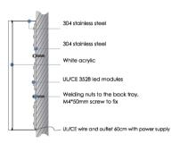
Front: 5MM/8MM thick acrylic Side: 1MM thick grade stainless steel
