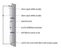
Front: 3MM thick acrylic Side: 3MM thick acrylic Back: Metal base
