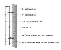
Front: 1MM thick 304 grade stainless steel Side: 1MM thick 304 grade stainless steel
